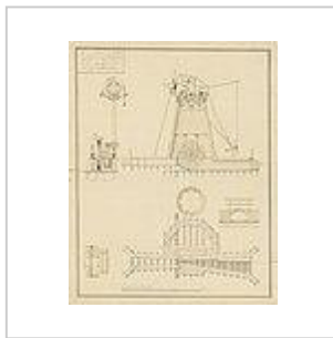
Technical drawing of a 1793 Dutch smock mill for land drainage
